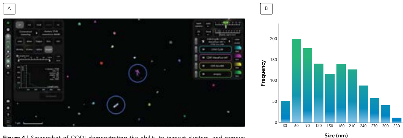
Figure 4 | Screenshot of CODI demonstrating the ability to inspect clusters, and remove localizations that do not correspond to set parameters (blue circles) (A). Histogram representing the sub-populations of EVs within a sample based on size analysis (B).
